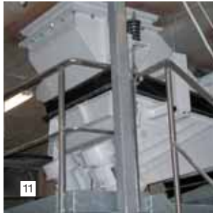
11 Regelbare Unwuchtrinne Unbalance motor feeder with stepless capacity adjustment
